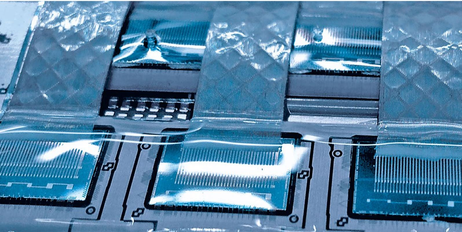
**Light-curing adhesives are primarily used in connection technology where rapid curing is required. These one-component products cure at room temperature within seconds after irradiation with UV light. This allows very short cycle times, even with large numbers of pieces.**
