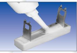
Applying 919 to a Hi-Power Resistor
