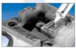
Bond-IT 7056AL Fills a Casting Before Re-Machining
