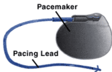
Figure 2. Generic Pacemaker and lead. Silicone adhesives can seal the lead to the pacemaker housing which is titanium.
