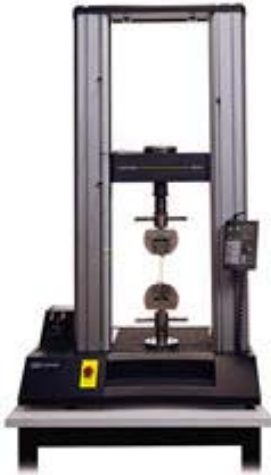
Figure 7. Instron 5500 Series Tabletop models for 450 lb to 11,250 lb capacities. New model updating the 1011.
