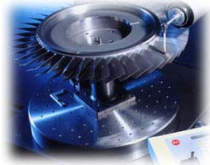
Figure 6. Titanium turbine blades during processing and fabrication.
