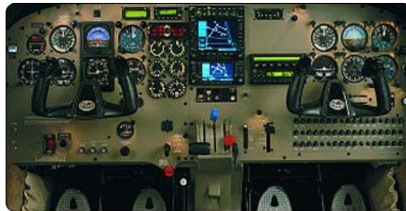
Figure 2. Aircraft cockpit showing Polyamide flight controls, PMMA displays, and polycarbonate & PEI flight consoles. Silicone adhesives can be used to seal the various components.
