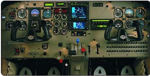
Figure 1. Aircraft cockpit showing Polyamide flight controls, PMMA displays, and polycarbonate & PEI flight consoles. Silicone adhesives can be used to seal the various components.
