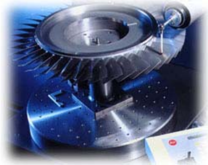
Figure 3. Titanium turbine blades during processing and fabrication.
