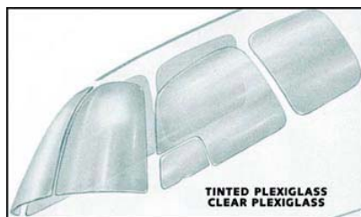
Figures 5. PMMA aircraft windshields are chosen for their excellent clarity and non-yellowing properties in outdoor environments. Silicones can be used to provide a seal around the windshield.
